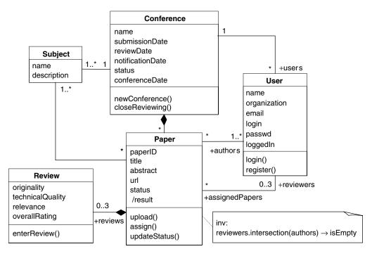
Figure 3-5 Class diagram for the reviewing system.
