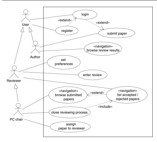
Figure 3-3 Use case diagram of the reviewing system.
