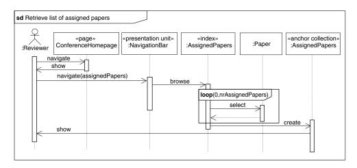
Figure 3-11 Sequence diagram for retrieving a list of assigned papers.
